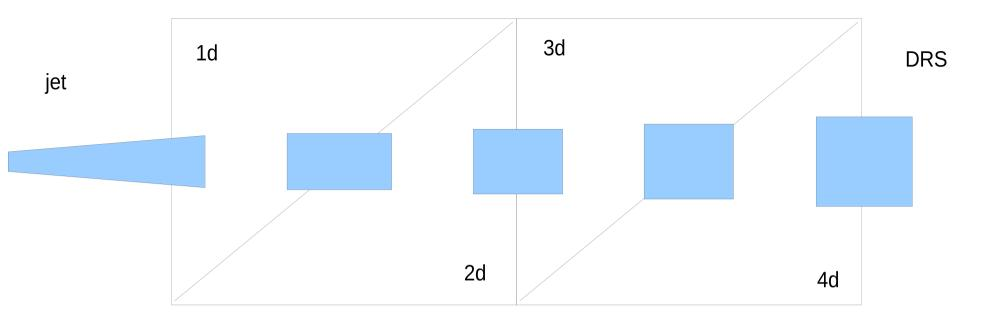
first aperture is conical and "re-entrant" (cone defined by DRS acceptance) remaining apertures can be tubes (diam. equal to DRS acceptance at largest distance)
